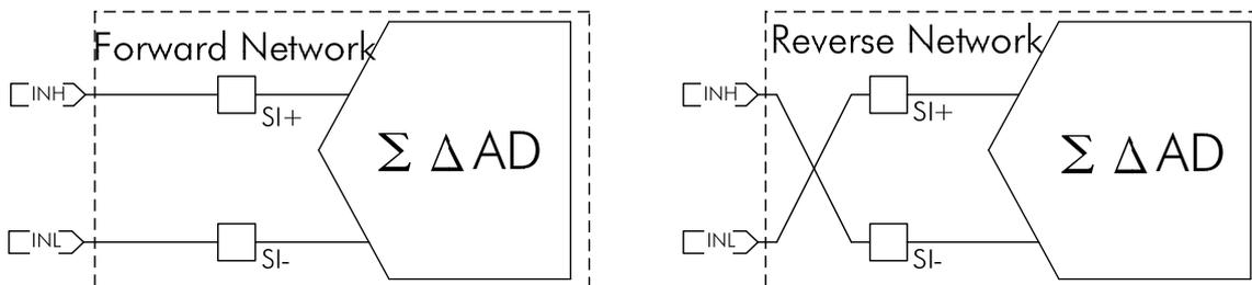
Figure 2 A/D Network Cross Diagram
