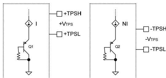
Figure 3 TPS Equivalent Circuit Diagram
