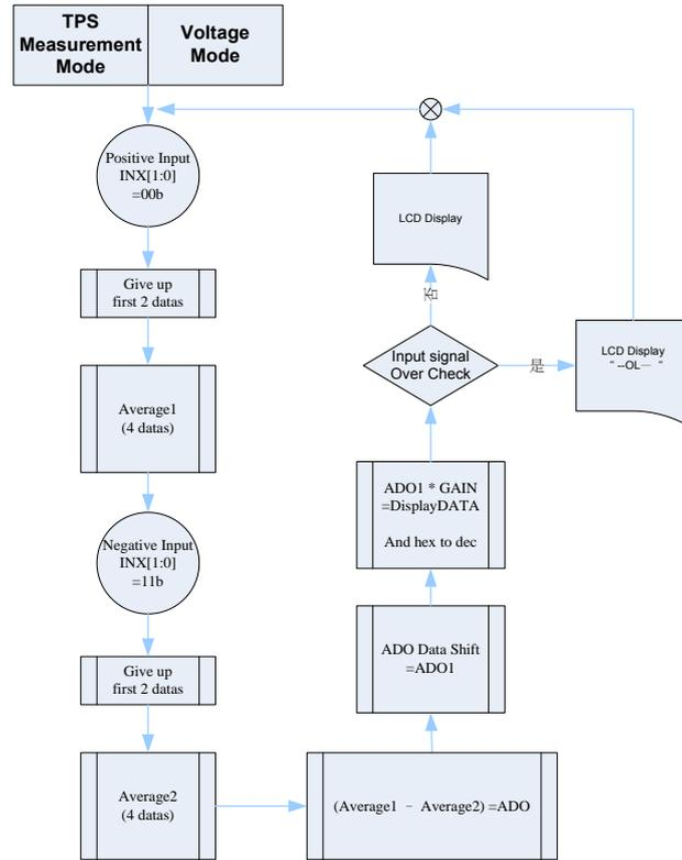
Figure 8 Measuring Flow
