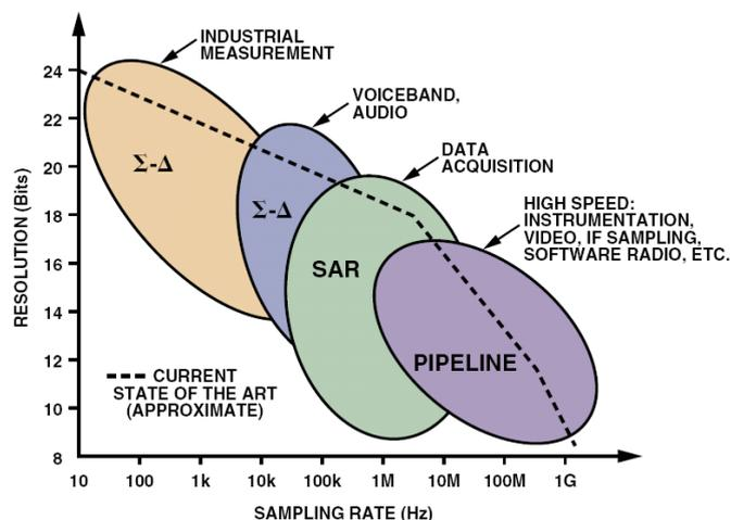
Figure 1 The Relationship of Different A/D Construction, Resolution and Sampling Rate [1]
