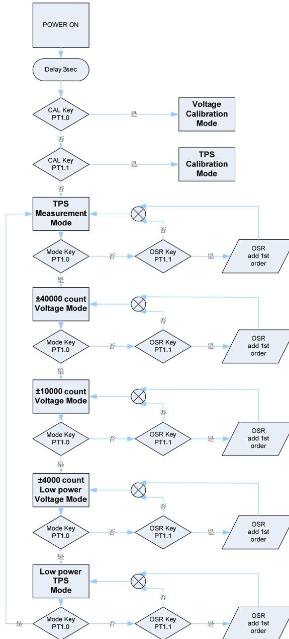
Figure 6 Flow Diagram
