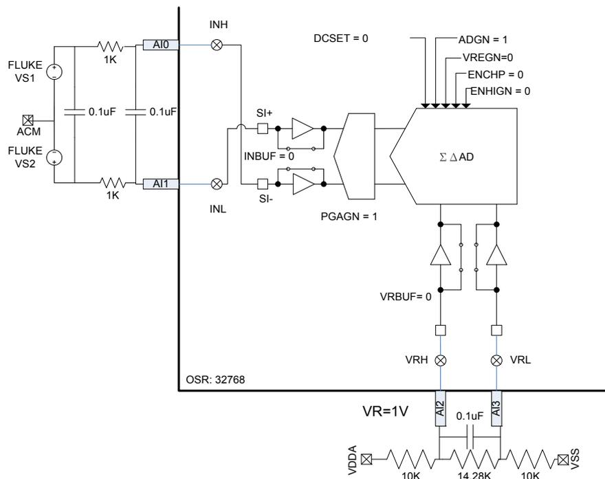
Figure 9 A/D INL Testing Circuit
