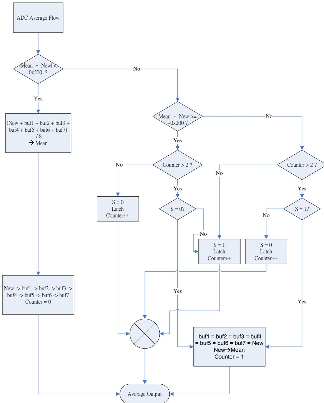
Figure 9 Digital Wave Filter Data Process
