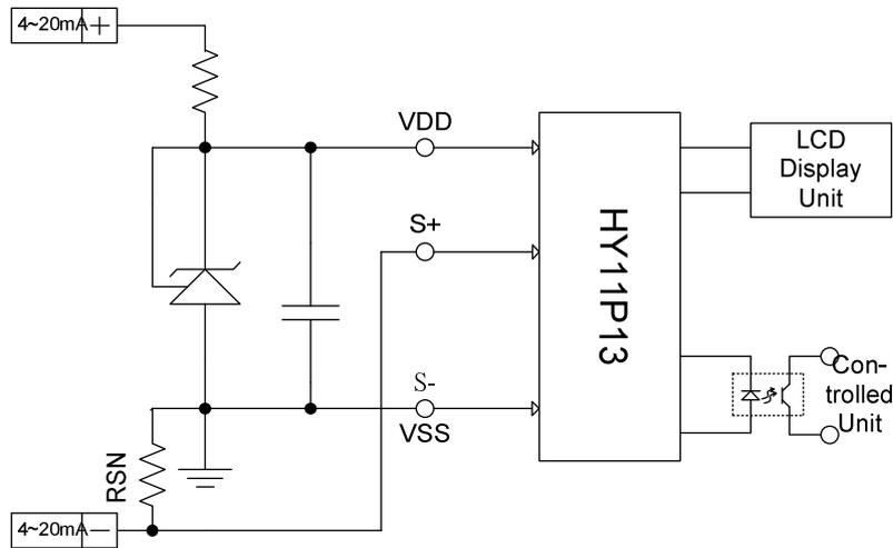
Figure 3 LCD Display Meter Controllers with HY11P13 Chip
