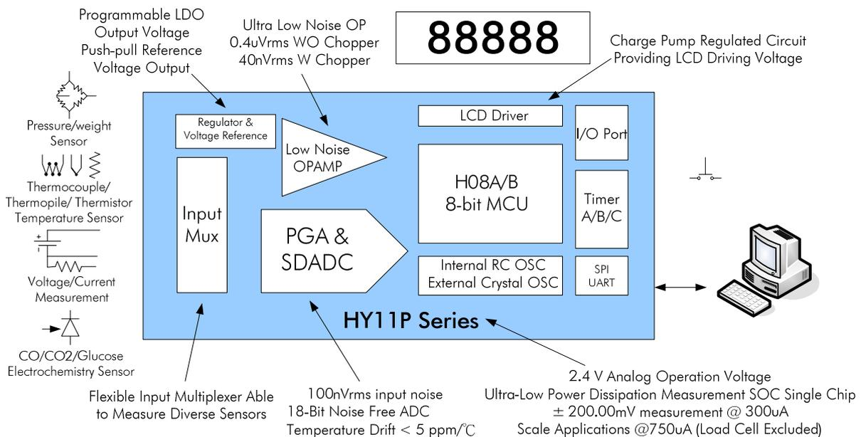
Figure 5 HY11P13 High Performance 8bit OTP Single Chip System
