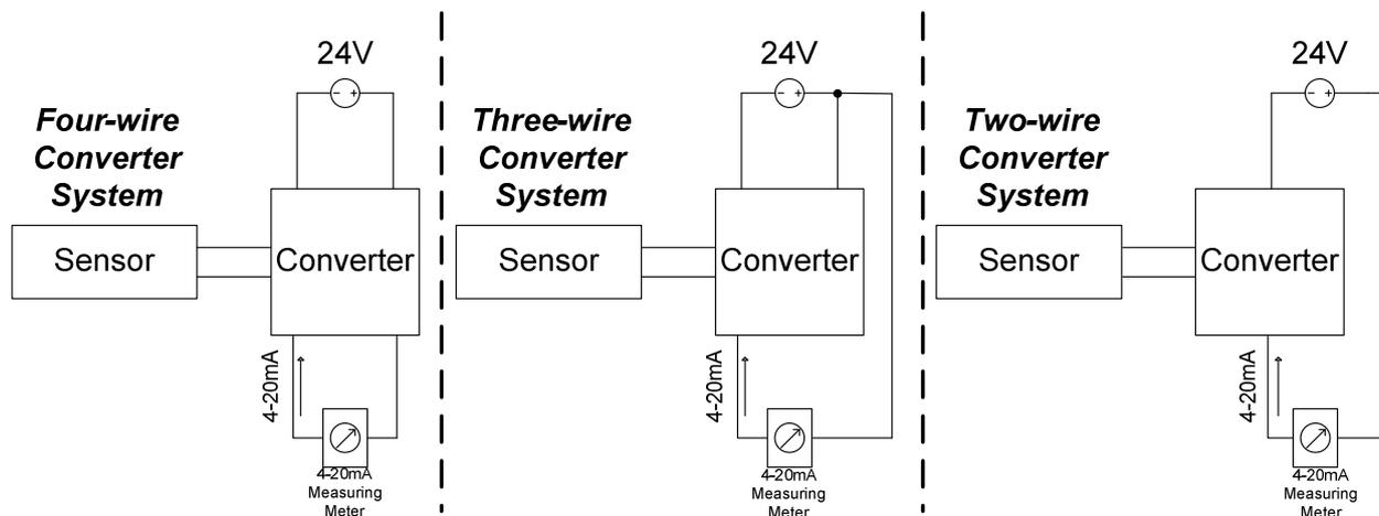
Figure 1 System Construction of Converters
