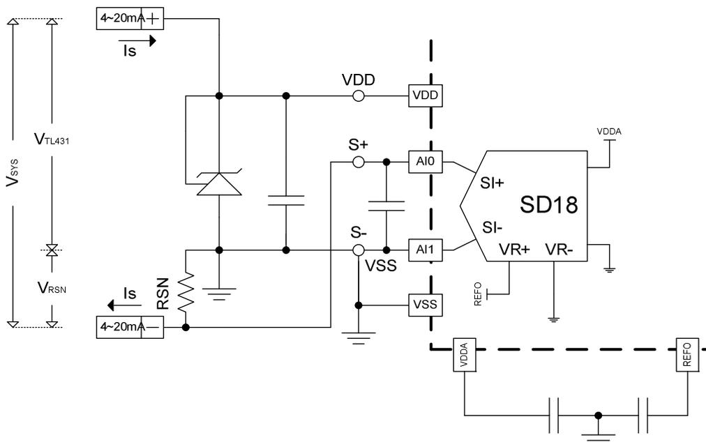
Figure 4 Measuring Construction of HY11P13 Chip
