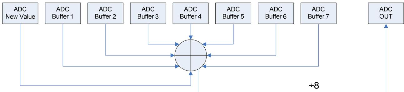
Figure 7 SD18 Output Data and Digital Wave Filter
