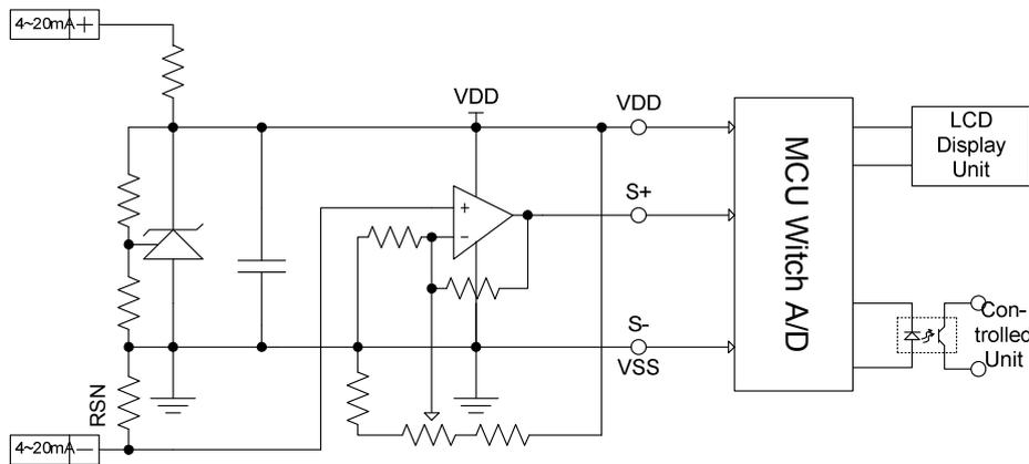
Figure 2 Ordinary LCD Display Meter Controller
