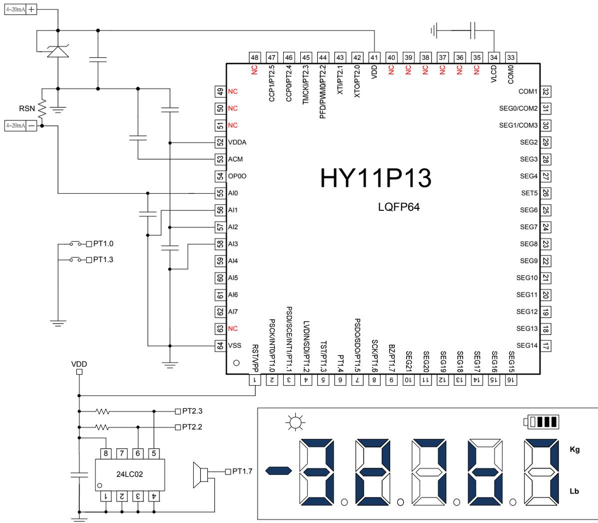
Figure 6 HY11P13 Application Circuit
