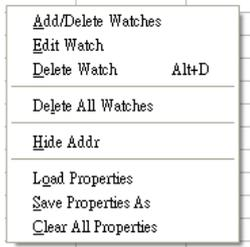
Monitor EQU defined Register or RAM, click the right key of mouse to select add-in monitored Register or RAM as Figure 3-15 described.
