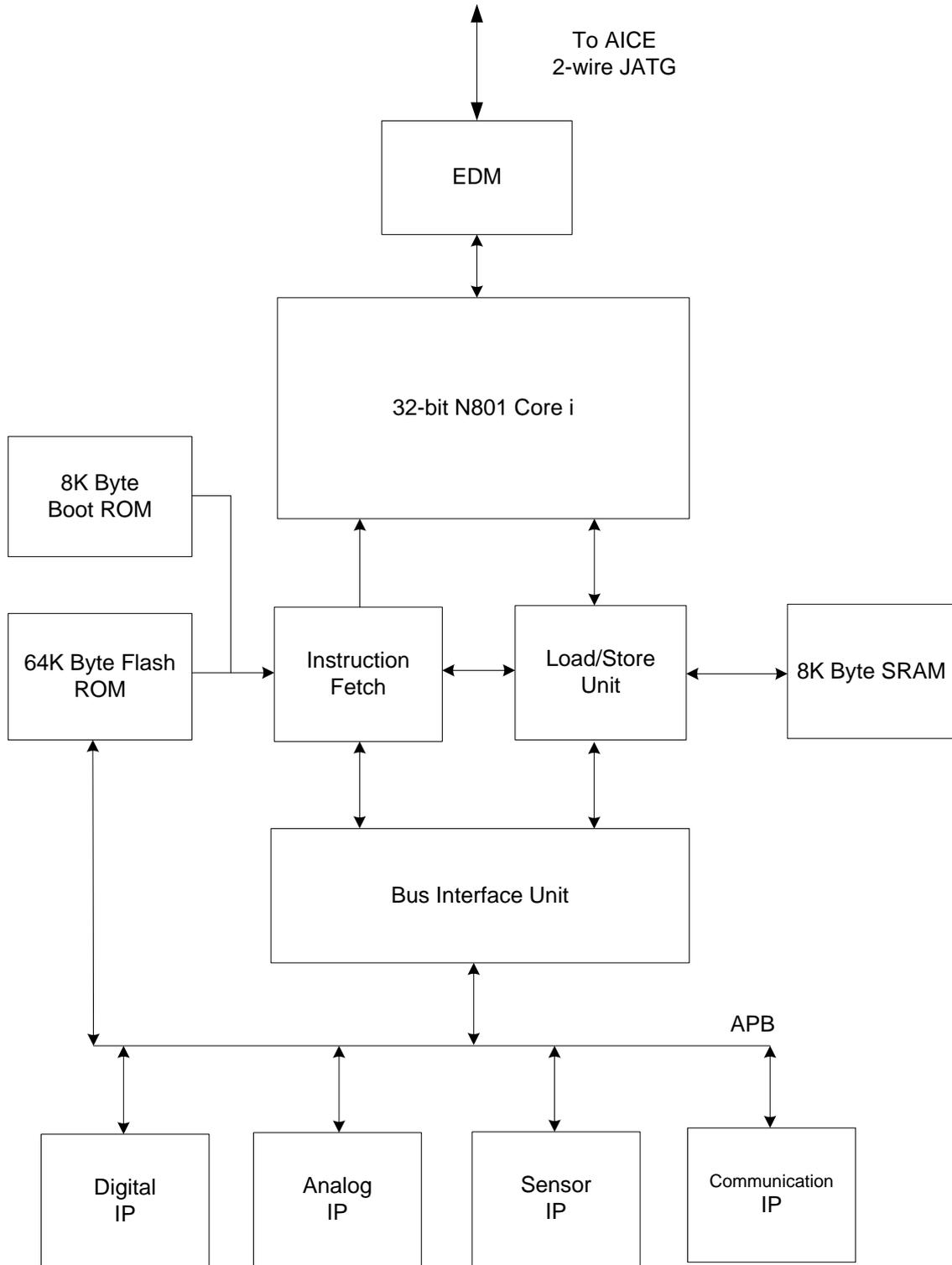
Picture2.2: IC Test Structure Diagram
