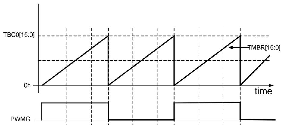
**FIG.10-11 Waveform schematic view and counting waveform schematic view of PWM mode G**
