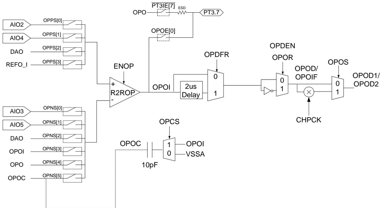
Fig 18-1 OPAMP function block diagram
