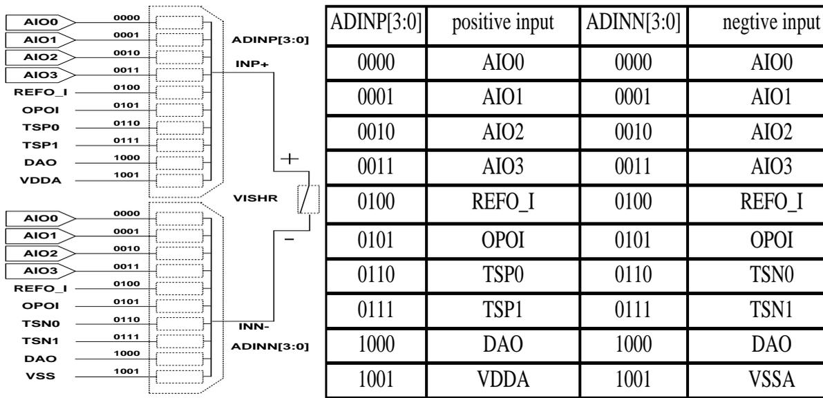
Figure 16-2 ADC signal input channel
