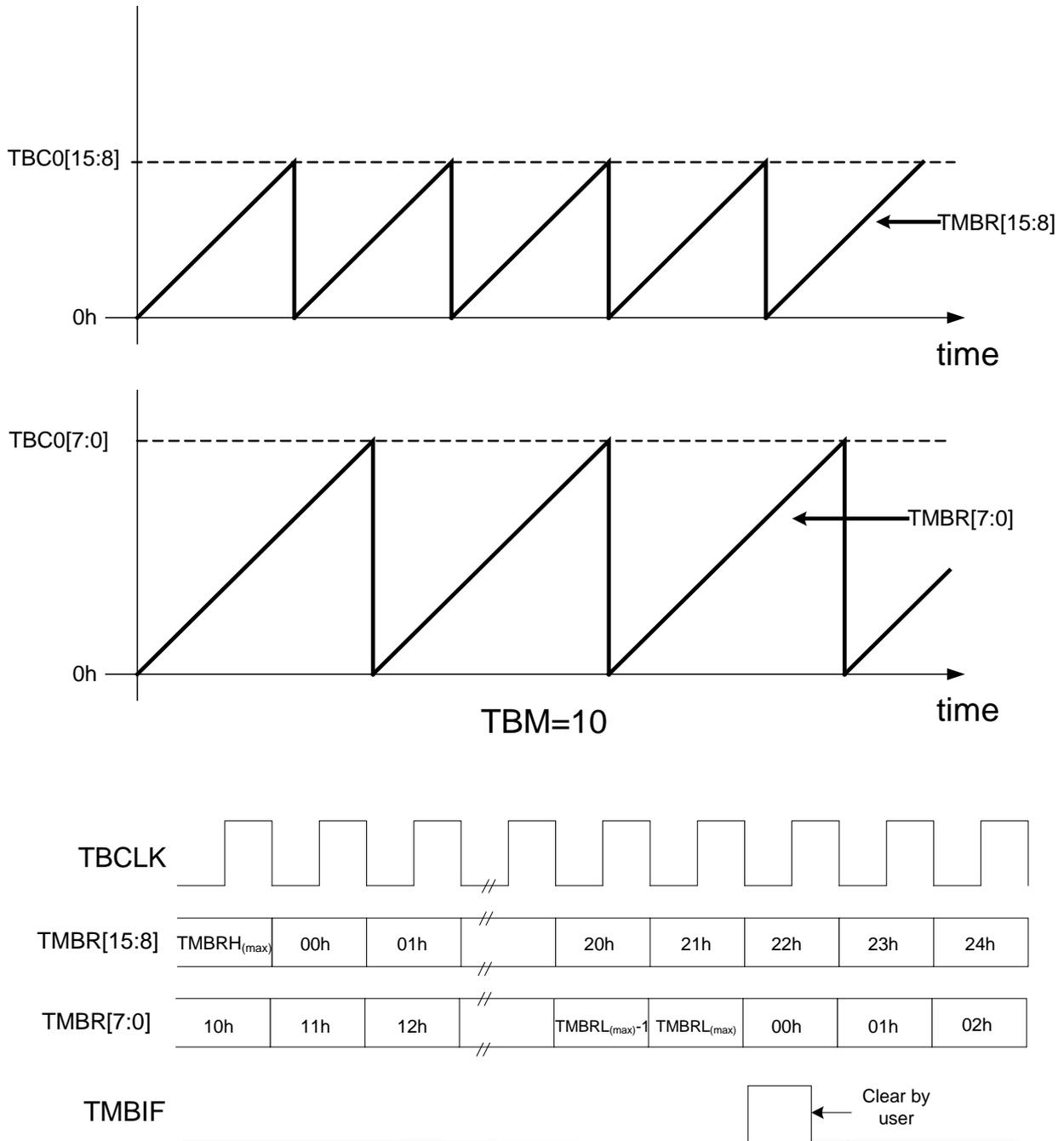
FIG. 10-4 Schematic view of counting waveform of counting method 2
