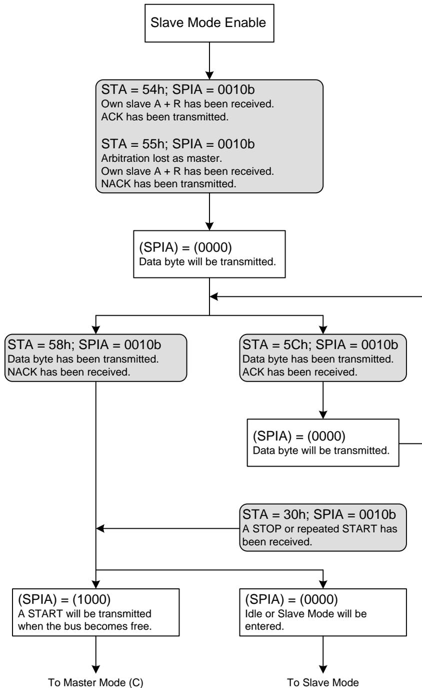
Fig 23-6 Slave Transmitter Mode
