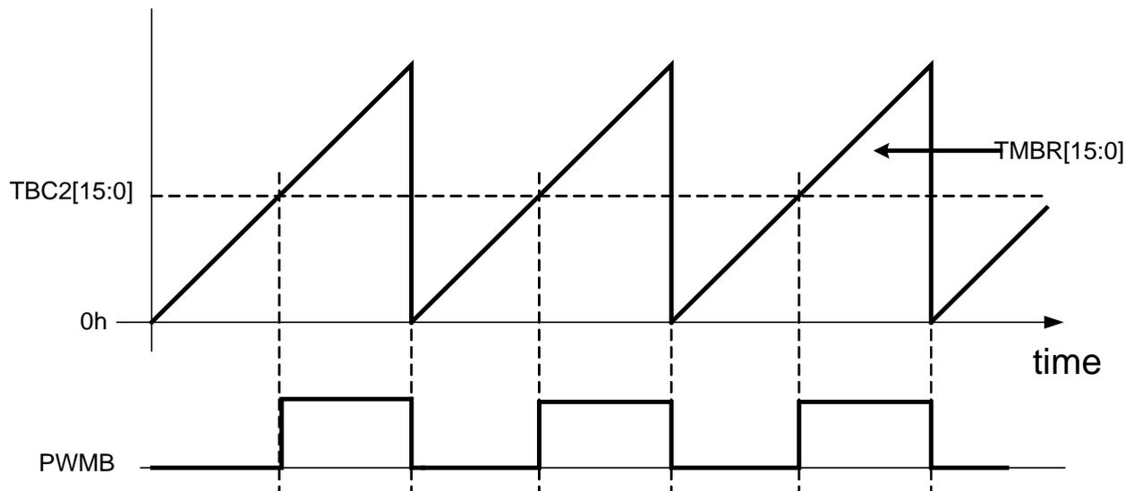
**FIG. 10-7 Waveform schematic view and counting waveform schematic view of PWM mode B**
