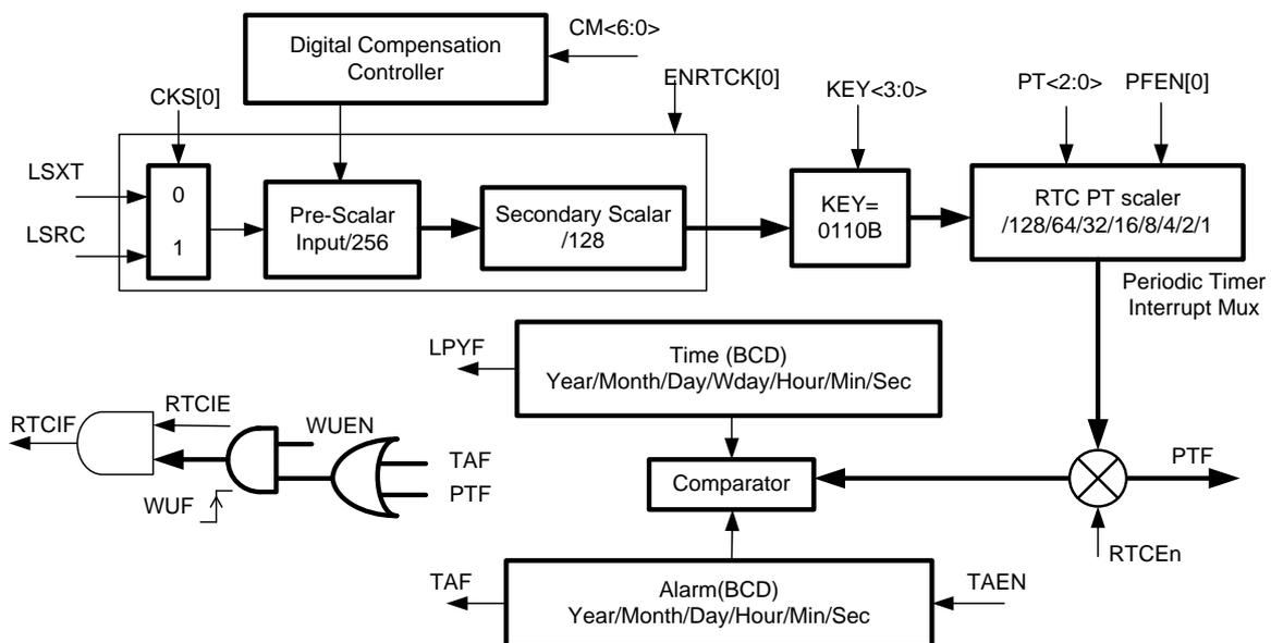
FIG. 24-1 RTC structure diagram
