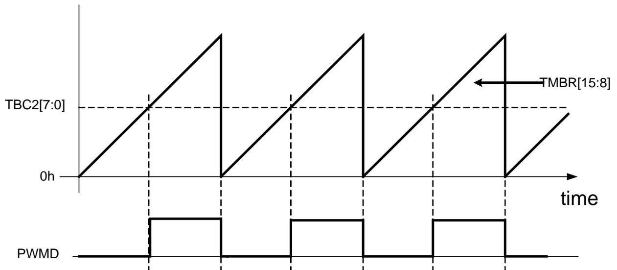
**FIG.10-9 Waveform schematic view and counting waveform schematic view of PWM mode D**
