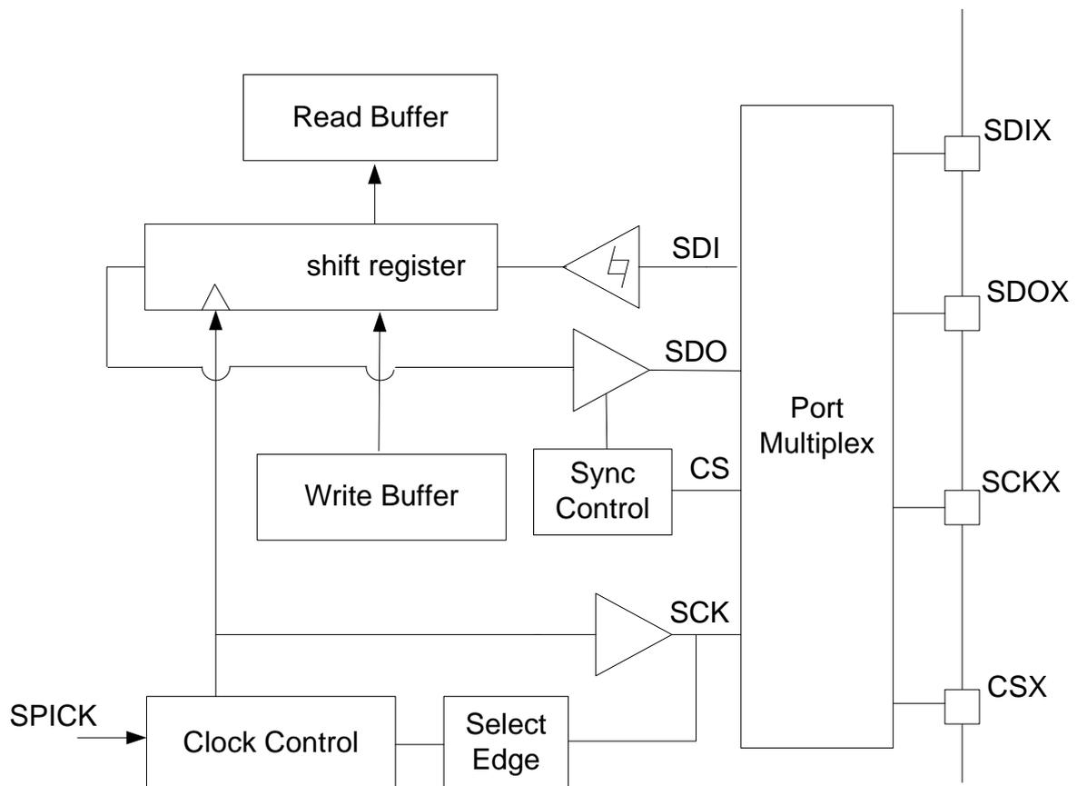
FIG. 21-2 SPI IO pin diagram
