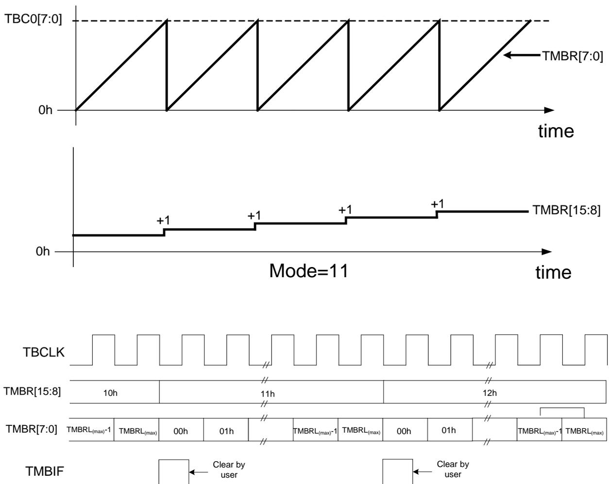
**FIG. 10-5 Schematic view of counting waveform of counting method 3**
