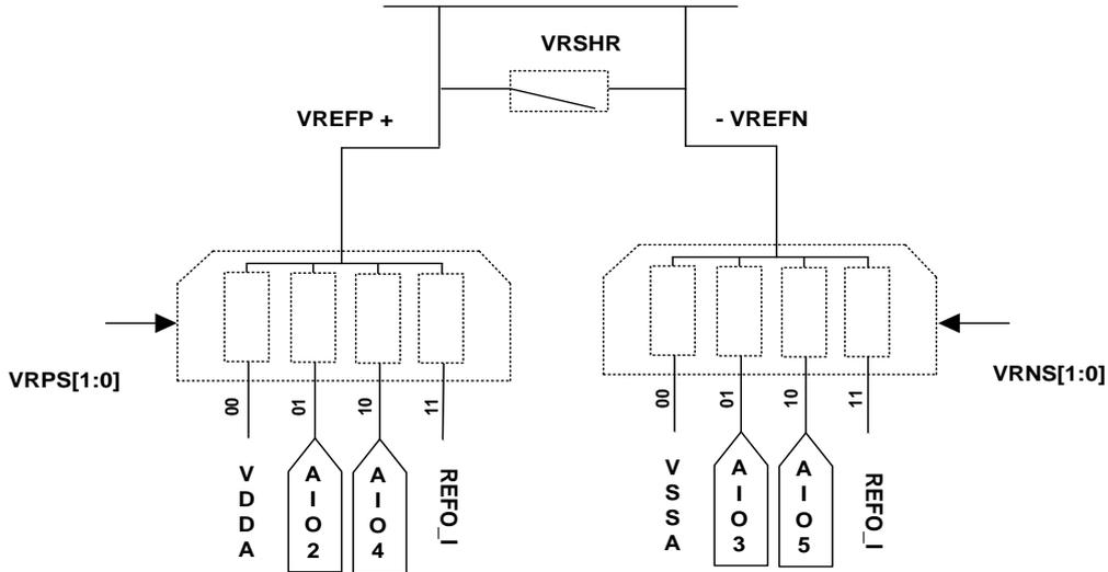
Figure 16-3 reference voltage input channels
