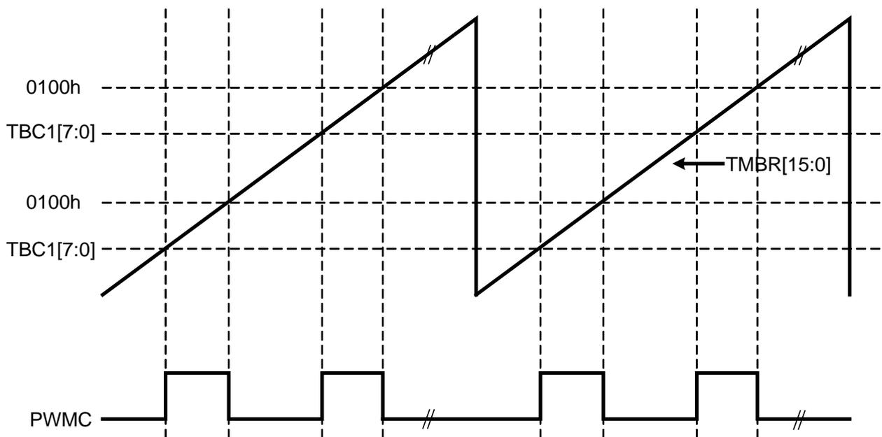
**FIG.10-8 Waveform schematic view and counting waveform schematic view of PWM mode C**
