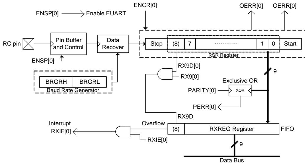
Figure 22-3 EUART 9-bits receiver block diagram
