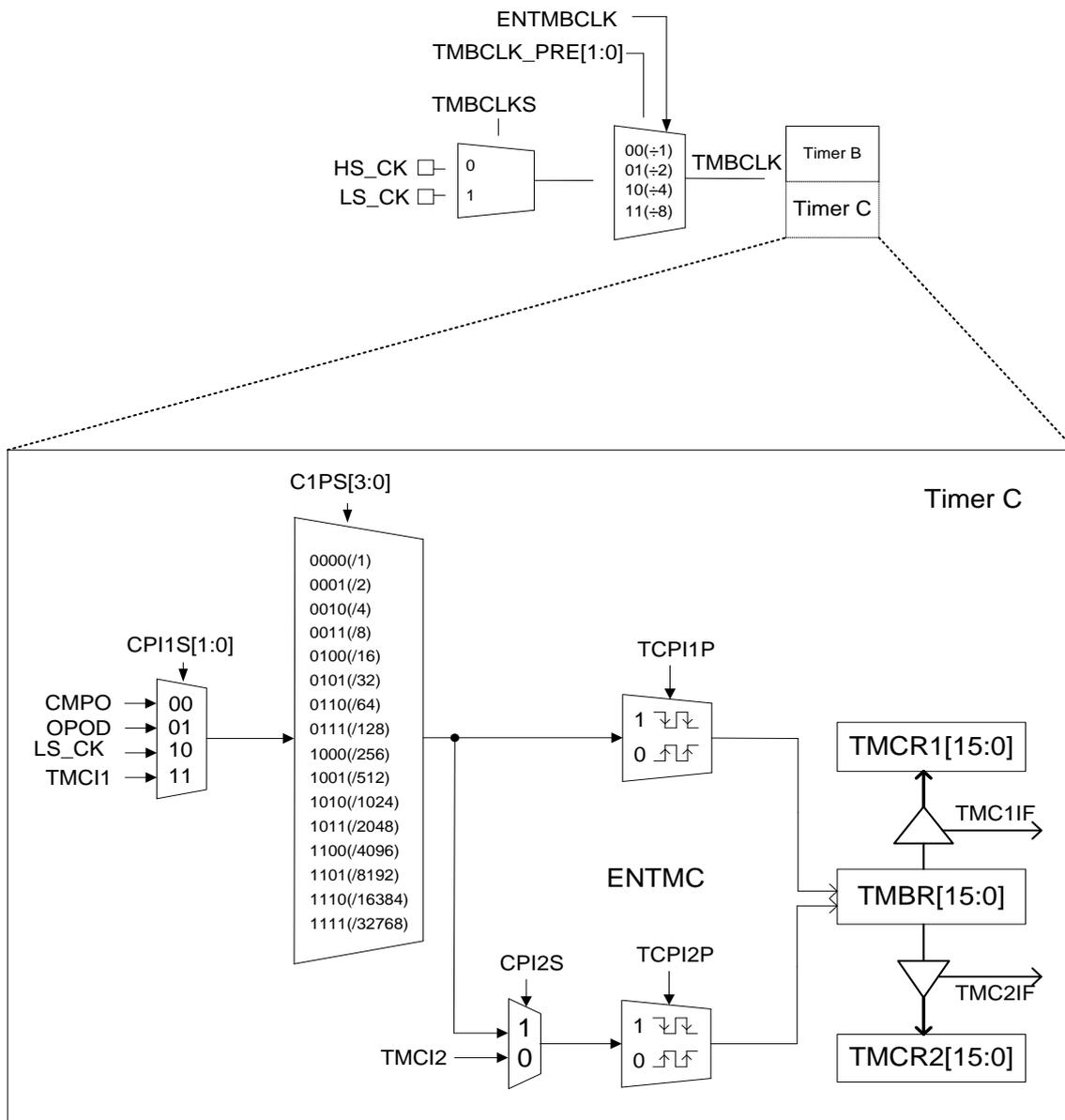
Fig. 11-1 TMC function block diagram
