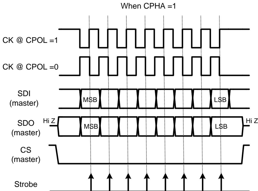
Note: SPI Interface when working in Master Mode, SCK operating frequency  $SPICK / 2$ .
