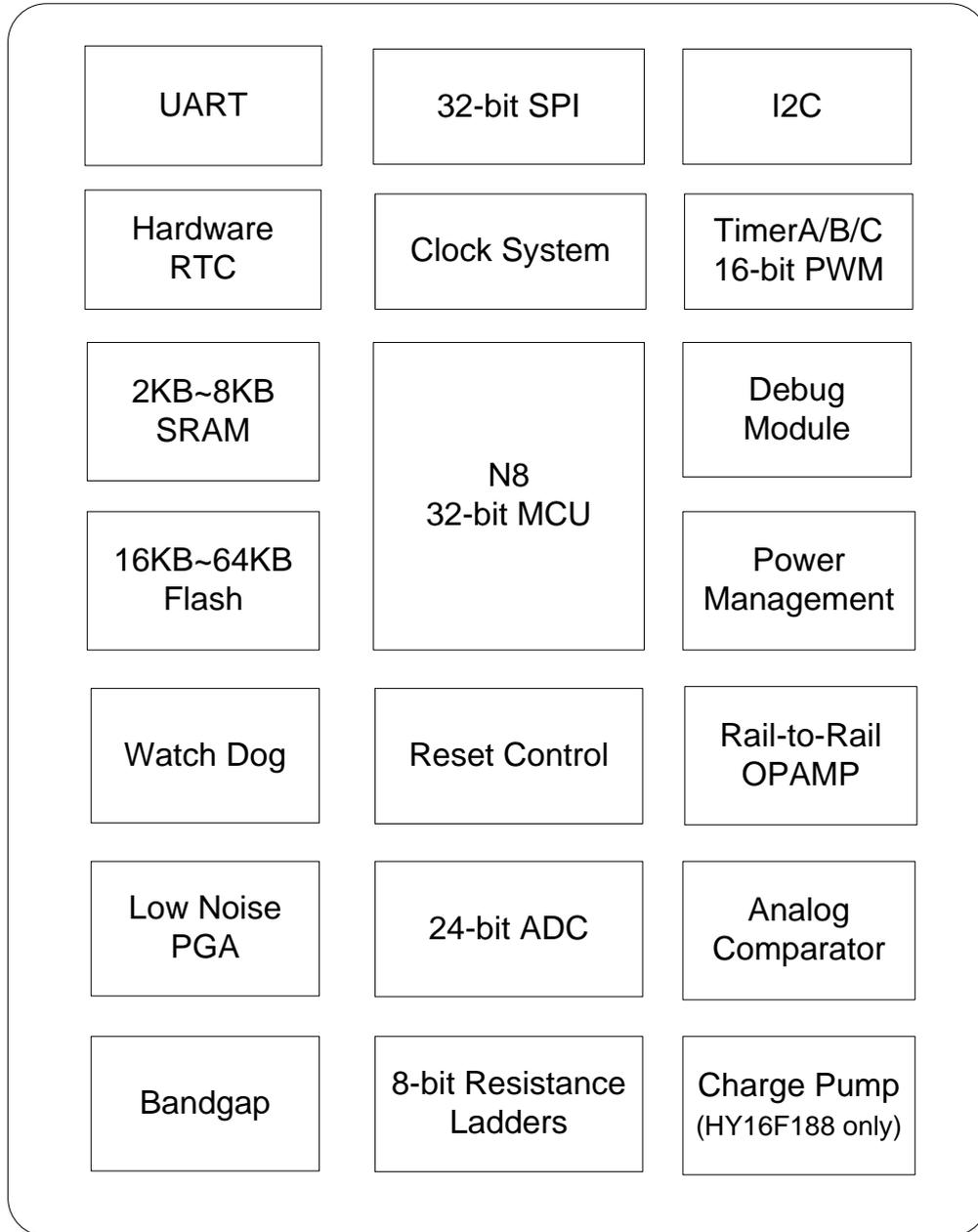
Picture 2-1: IC Function Structure Diagram
