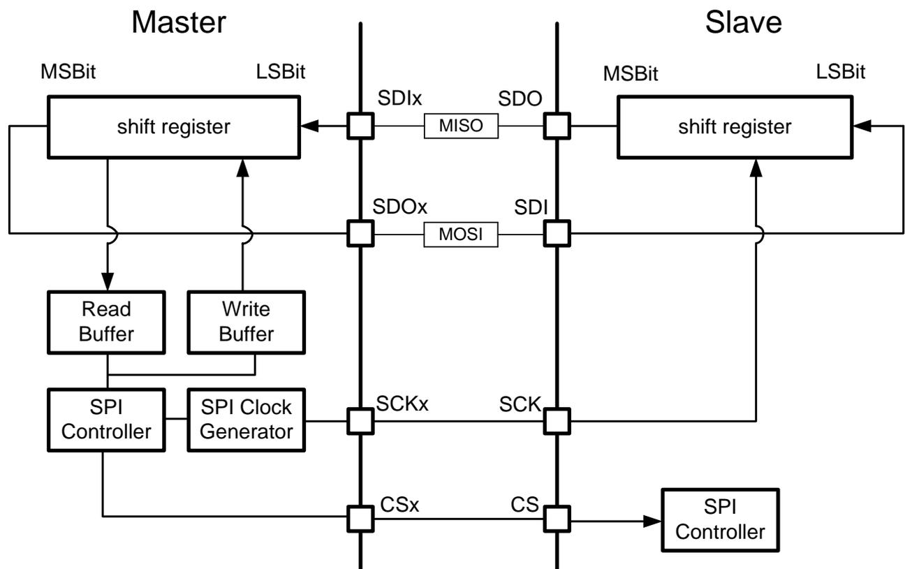
FIG. 21-1 Serial communication SPI structure diagram
