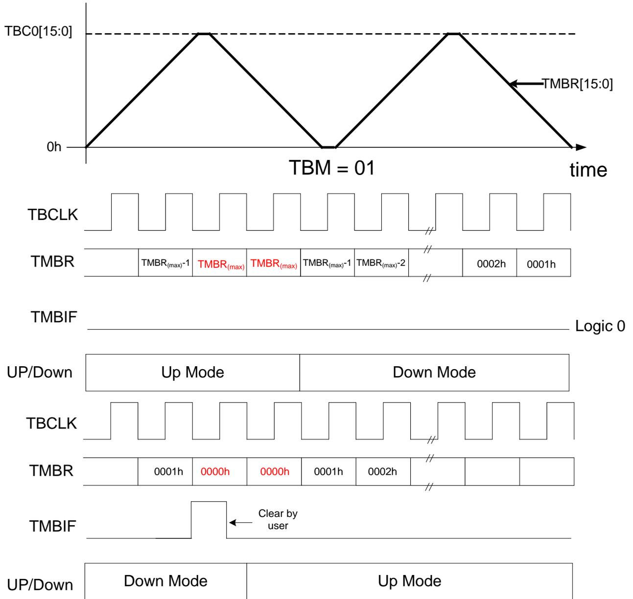
FIG. 10-3 Schematic view of counting waveform of counting method 1
