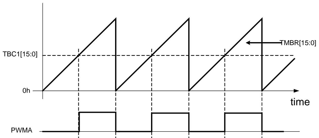
**FIG. 10-6 Waveform schematic view and counting waveform schematic view of PWM mode A**
