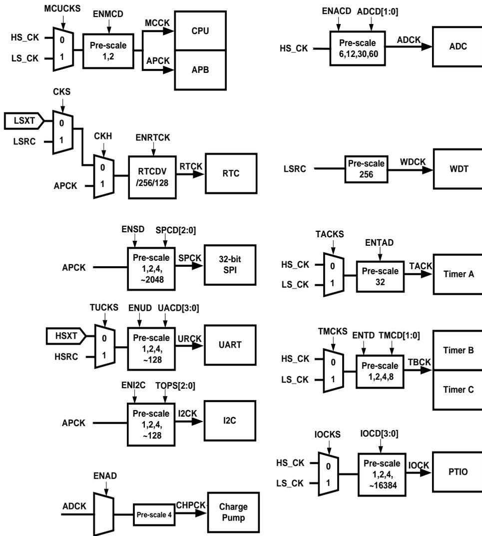
Table 6-2 External peripheral operating frequency configuration diagram
