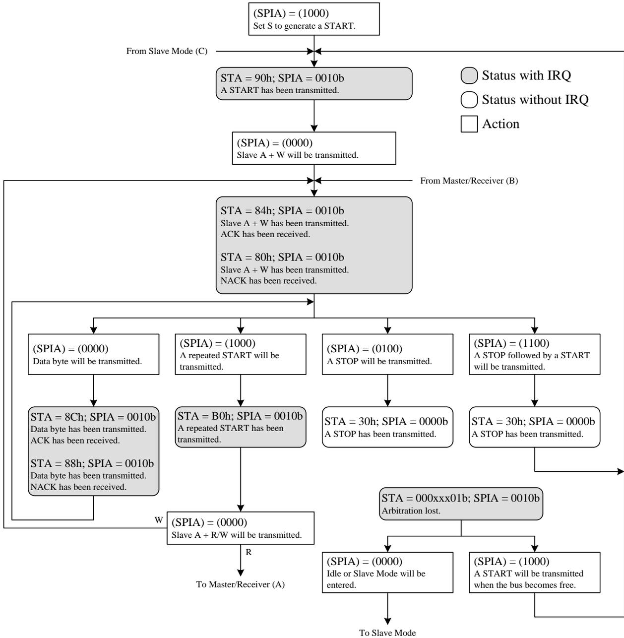
Fig 23-4 Master Transmitter Mode
