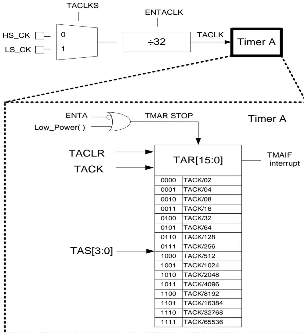
FIG. 9-1 Timer A block diagram
