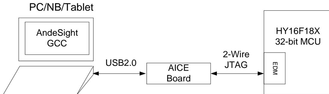
FIG. 3-4 Chip development connection diagram
