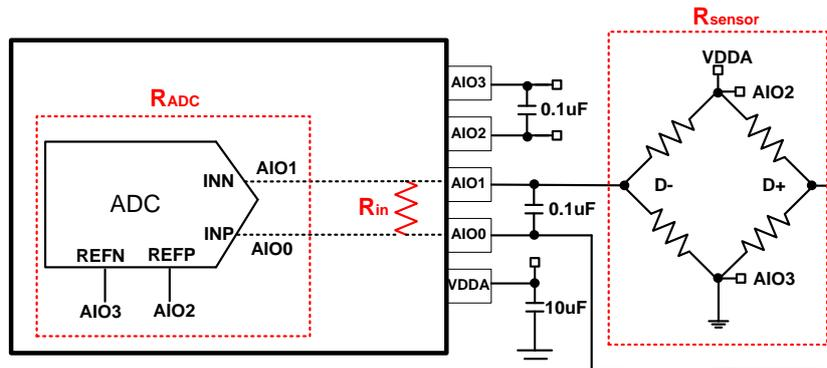
( $R_{in}$ ) and ( $R_{ADC}$ ) and ( $R_{sensor}$ ) relationship is:  $R_{in} = R_{sensor} // R_{ADC}$
