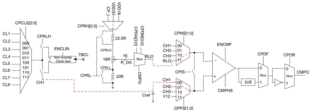
FIG. 20-4 Touch button connection diagram (One possible configuration)
