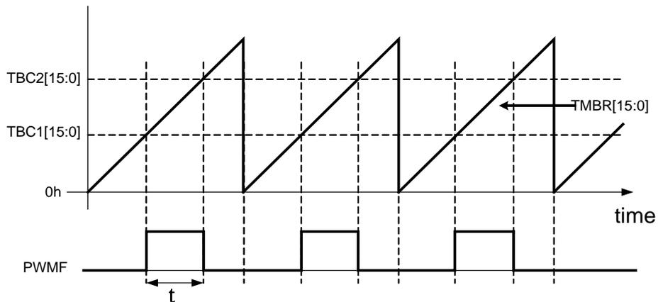
**FIG.10-10 Waveform schematic view and counting waveform schematic view of PWM mode F**
