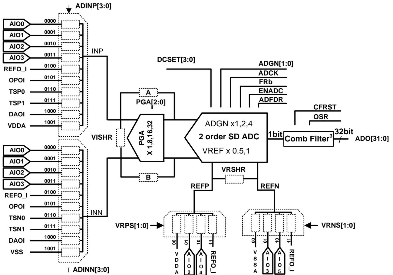
Figure 16-1 ADC function block diagram
