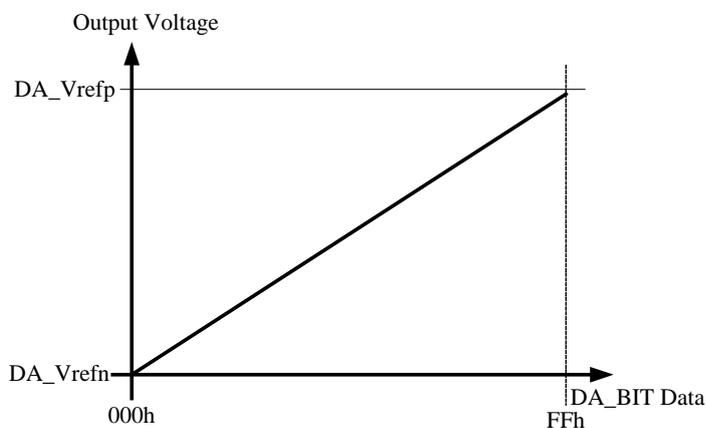
Fig 19-1 8-bit resistor ladders transfer function
