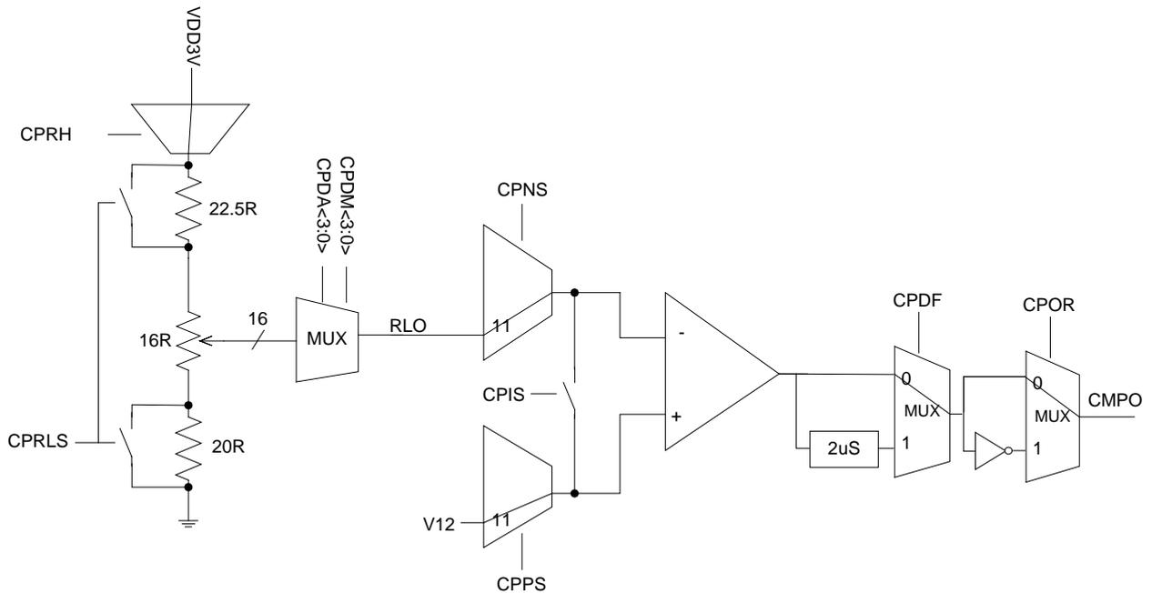
**20.4.2. CMP is used to measure capacitors**
