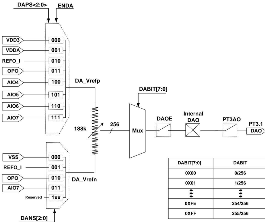
Figure 19-2 8 bit Resistance Ladder function block diagram
