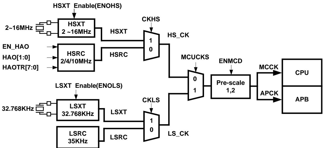
Table 6-1 CPU operating frequency source configuration diagram
