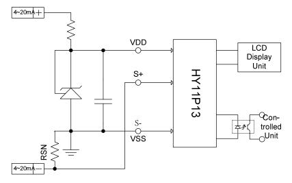
Figure 3 LCD Display Meter Controllers with HY11P13 Chip
