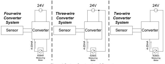
Figure 1 System Construction of Converters
