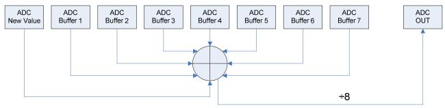
Figure 7 SD18 Output Data and Digital Wave Filter
