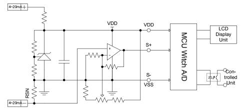
Figure 2 Ordinary LCD Display Meter Controller
