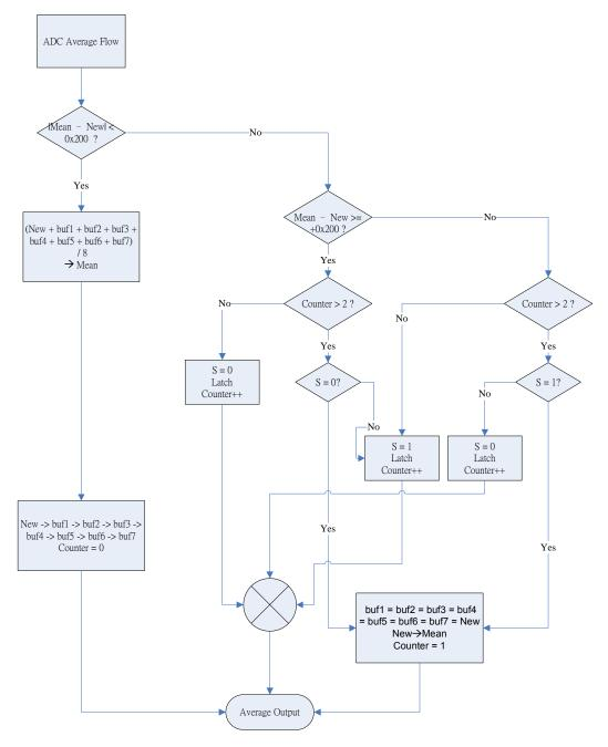
Figure 9 Digital Wave Filter Data Process
