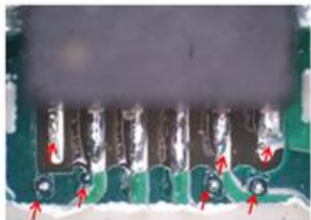
Incomplete reflow of solder paste
