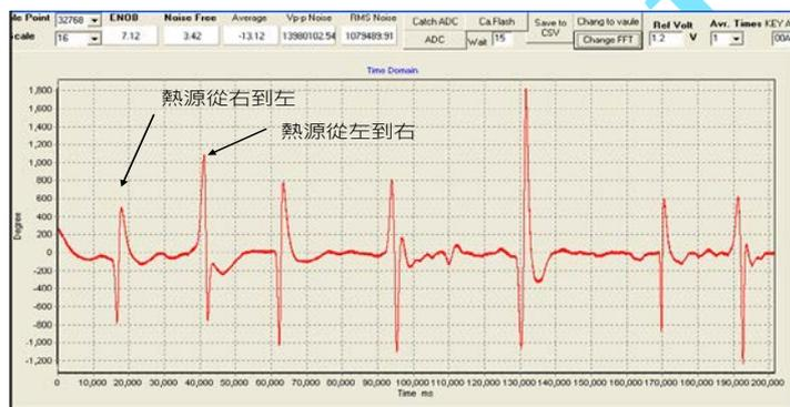
FIG. 5 The ADC output is 1KHZ, and the protrusion waves are the signals taking place when a heat source passes through.
