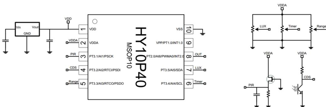
FIG. 4 Application circuit of HY10P40 PIR detector
