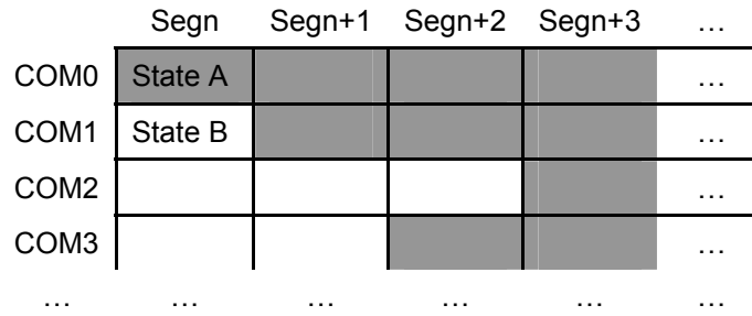
Figure 20 1/3-bias, 1/4-duty LINE Inversion
