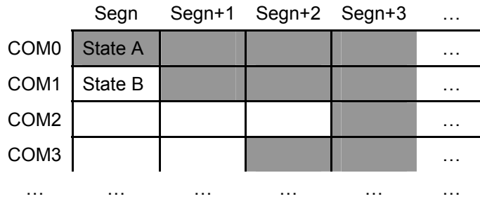
Figure 24 1/2-bias, 1/4-duty LINE Inversion
