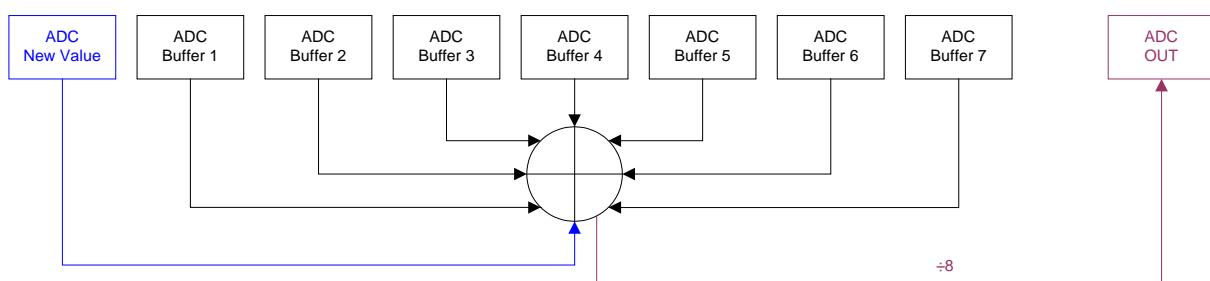
After ADC average output, ADC new value is transmitted to Buffer 1, from buffer 1 to buffer 2,..., and from buffer 6 to buffer 7, as demonstrated in the illustration below.
