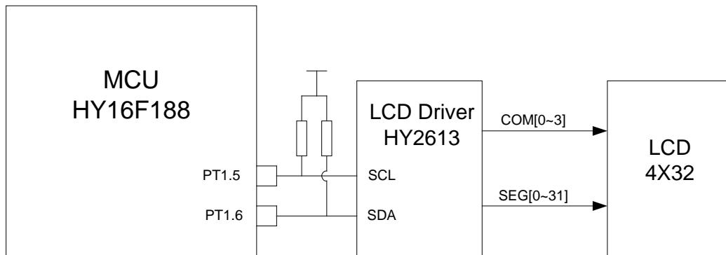
Through communication between IIC and LCD driver, MCU circuit becomes extremely easy, and convenient for operation. Once data is delivered to LCD driver HY2613, MCU can deal with other things, with information update becoming easy.
