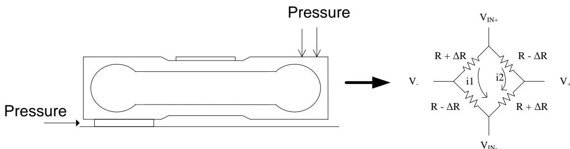
Voltage variation at both terminals in signal generated from  $\Delta R$  variation is:
