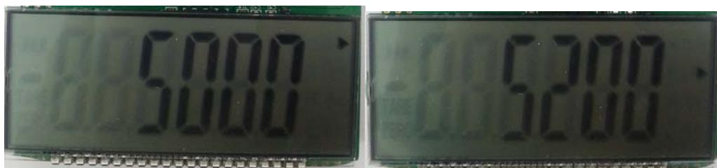
Procedure 4: Zero Calibration. Under this moment, MCU will automatically catch ADC value to determine its stability. After stabilization, the next step will be accessed. If stabilization fails to show up, user can gain access to the next procedure by clicking Touch Key 4 to force value catching.
