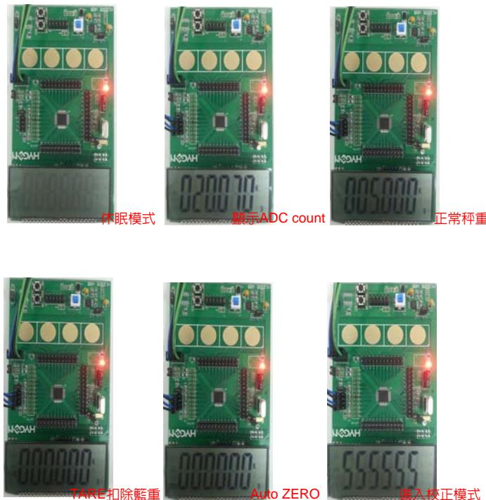
TARE will be displayed under basket weight elimination, while ZERO will be displayed under Auto zero. A backward counting from 5 to 1 will manifest before accessing calibration mode.
