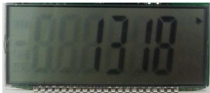
Procedure 7: Initial calibration in procedure 7 is touch key calibration. Untouched value will be caught at first, with LCD display altering between 888888 and 000000. Please don't click touch key under this moment. The next procedure will be automatically accessed upon completion.
