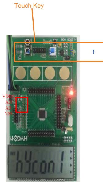
Under measurement mode, pressing Touch Key 1 will turn off LCD display and access sleep mode, pressing Touch key 2 converts LCD display from g to AD count, pressing 3 eliminates basket weight, while pressing Touch key 4 accesses calibration mode.
