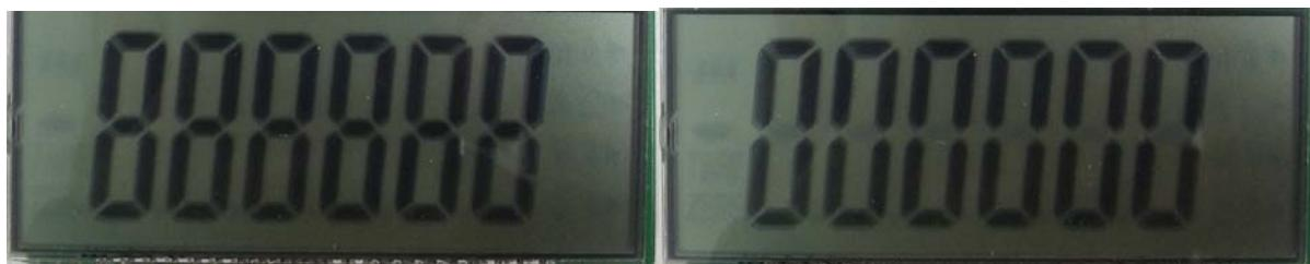
Procedure 8: Touch key threshold catching. 99XXXX will be displayed on the LCD screen. If XXXX takes form in numbers, please click the corresponding touch keys. After the four touch keys has been touched, meter will automatically return to measurement mode from calibration mode.
